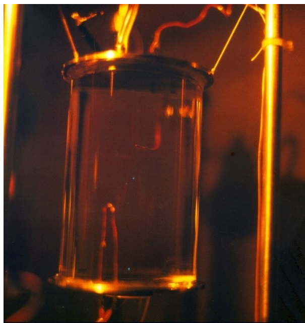
Figure 19: A standing sound wave with a frequency of 40,000 cycles per second generates 40,000 flashes of light per second that can be seen with the unaided eye. The blue/purple dots are the micron-sized spots formed in water by imploding bubbles. Courtesy : Photograph by Ed Kashi
